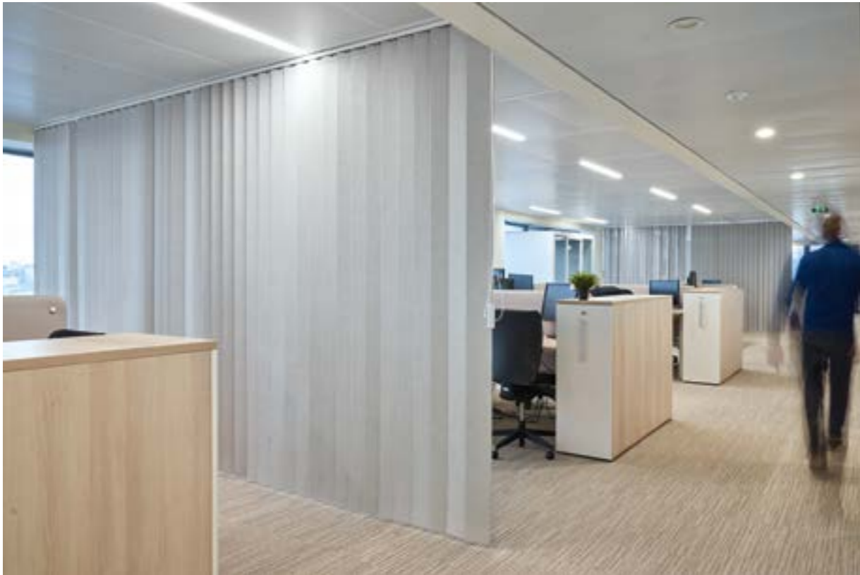
Velio acoustic blinds suspended from the ceiling to visually partition work areas while also improving the acoustics. Offices of PRO BTP insurance company in Montreuil, east of Paris, in 2022.
